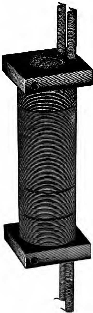
FIG. 87.—A telephone induction coil of usual size, showing the laminated core and the attachments of the primary and secondary windings.
